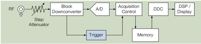
The oscilloscope-based acquisition system in the MDO4000 also provides an inherently triggered acquisition system. Data is acquired in a single contiguous time-domain record. This record is then digitally downconverted to the desired span and then run through a DFT to convert it to the frequency domain. As a result, the entire set of frequency domain data displayed for a single acquisition is time consistent – it comes from the same triggered data record.
