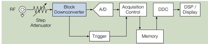
Because of the oscilloscope-based acquisition system in the MDO4000, a straightforward block downconverter is used to bring the frequency span of interest into the range of the A/D converter.
