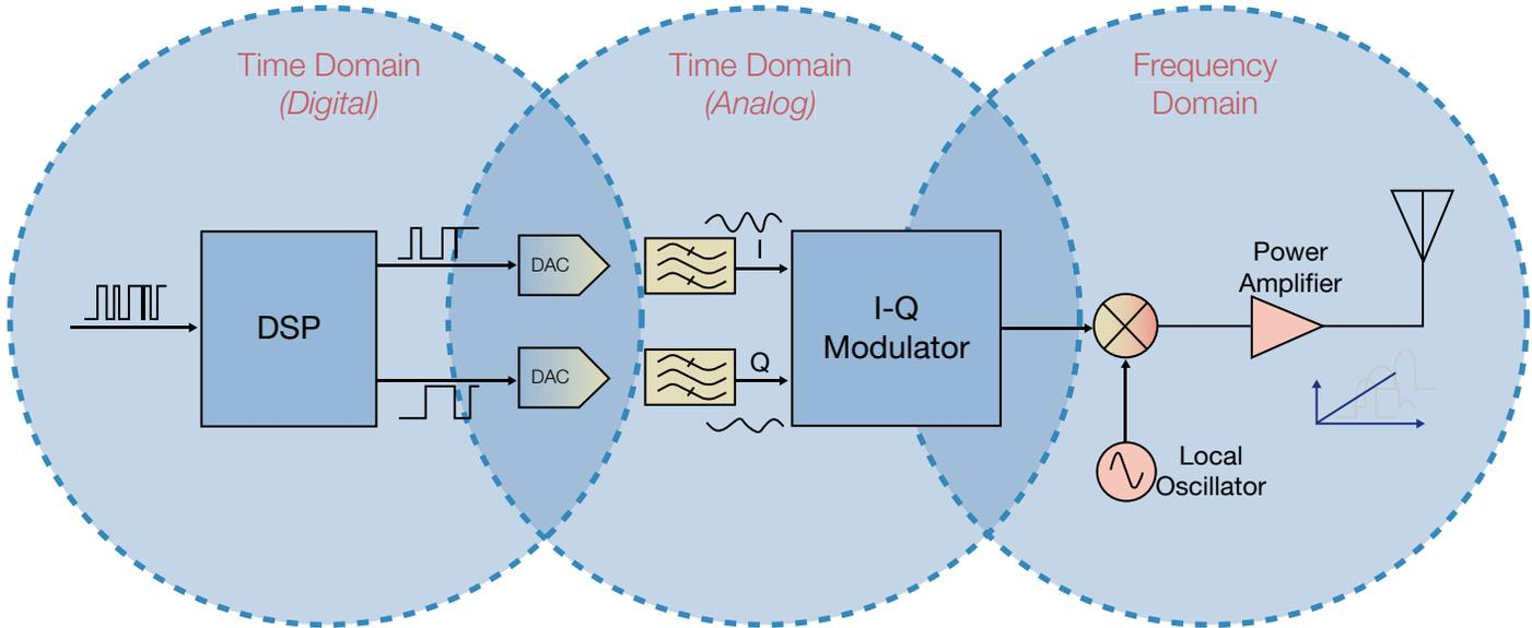
Figure 1. Modern Wireless Transmitter simplified block diagram.
