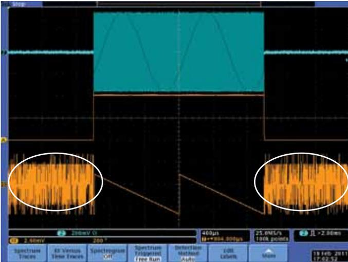
Figure 43. Phase vs. Time, Unblanked.
