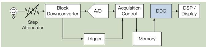
A common and computationally efficient way to represent bandpass signals is to use the complex baseband representation of the waveform. The first step in converting to the frequency domain is to perform Digital Downconversion on the raw RF time domain record. This process achieves three things:
