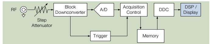
Another use for the IQ data is in generating RF Time Domain Data. Recall, from Digital Downconversion, that the IQ data is merely a Cartesian representation of the signal plotted as a vector in the imaginary IQ data plane. As such, the IQ data can be transformed as shown in Figure 42.
