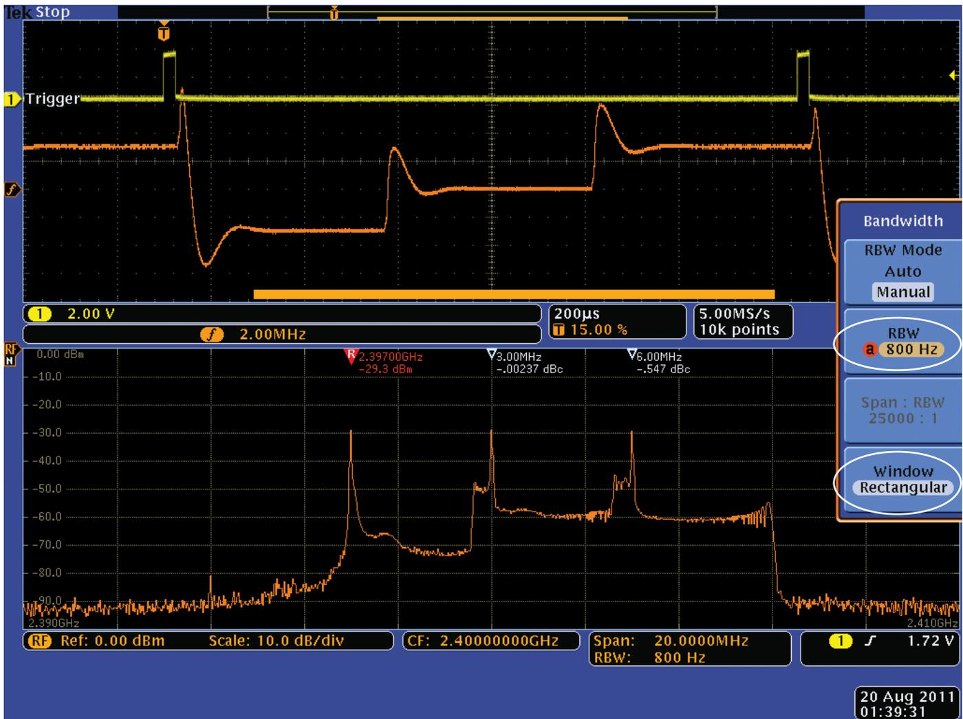
Figure A6. Rectangular Window in 750 Hz RBW.
