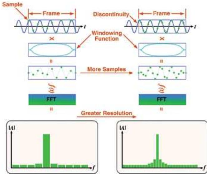
Figure 41. Increased time samples improves frequency domain resolution.
