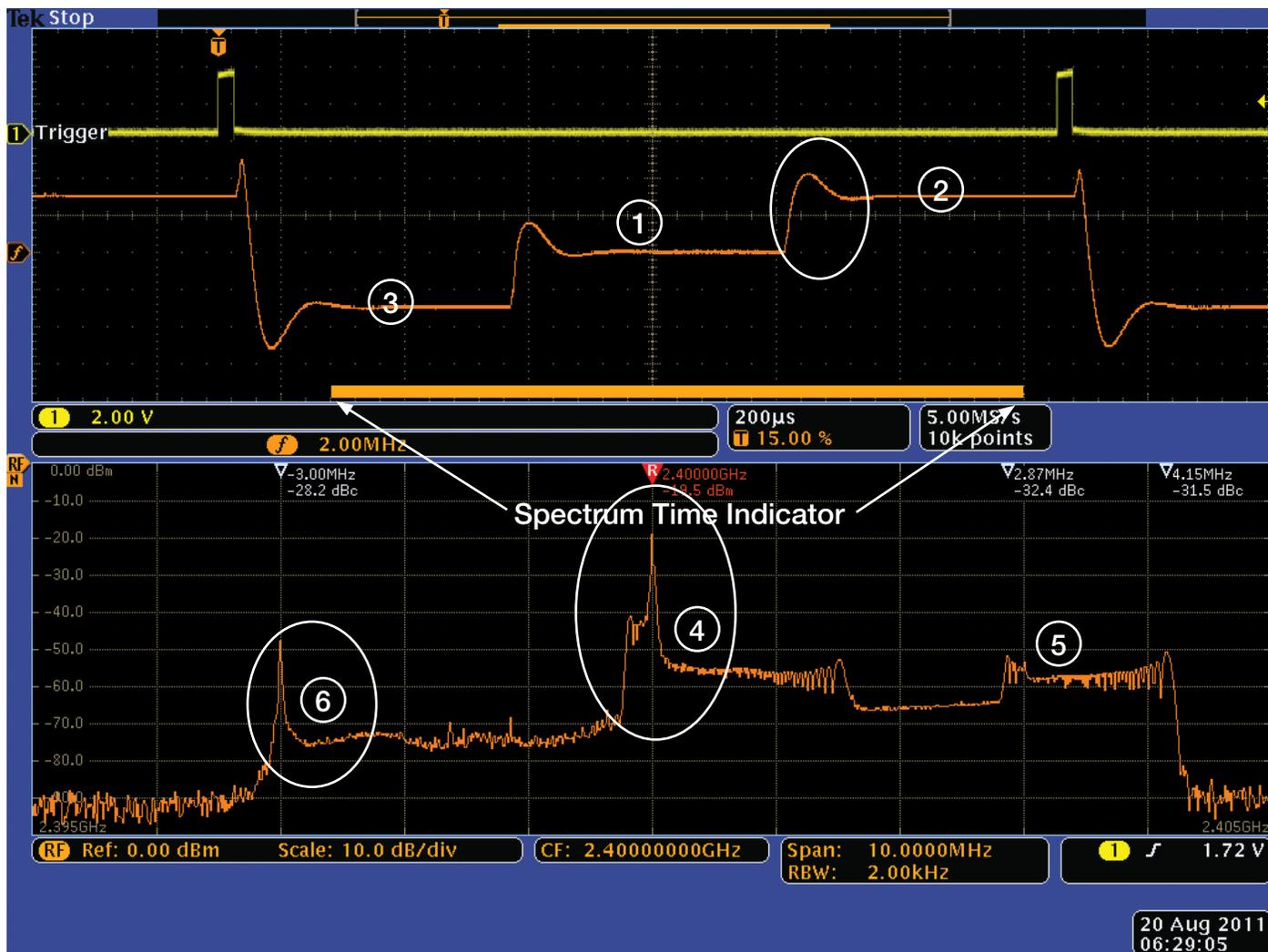
Figure 17. Spectrum Time Indicator.
