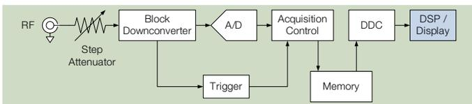
Figure 40 illustrates the process of generating the spectrum trace for display.
